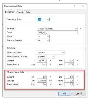
In order to enter the currents of all conductors in different ways, up to 4 measured values (L1, L2, L3 and N) are required on the same terminal.
