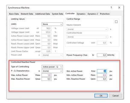
This special reactive power controller is particularly important when decentralized infeeders are involved. The network operator mostly requires here a reactive power infeeder adjusted to the active power.
