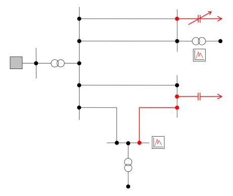
This shows a network element group with the following elements (shown in red in the illustration): Line, capacitor with fixed power value and capacitor with variable power value in 3 tap positions and actual controller position 2.
