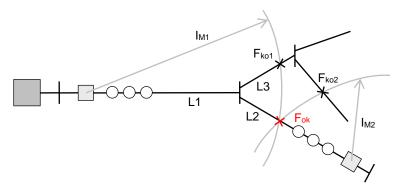
In the example above, the actual fault is located on line L2. The percentage current deviation at this fault position has a value of about zero. The percentage deviation at all other fault positions is considerably higher.
