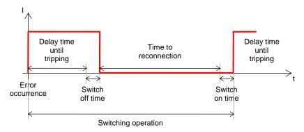
This switching operation is repeated depending on the configuration. Three switching operations produce the following curve characteristic for the section.
