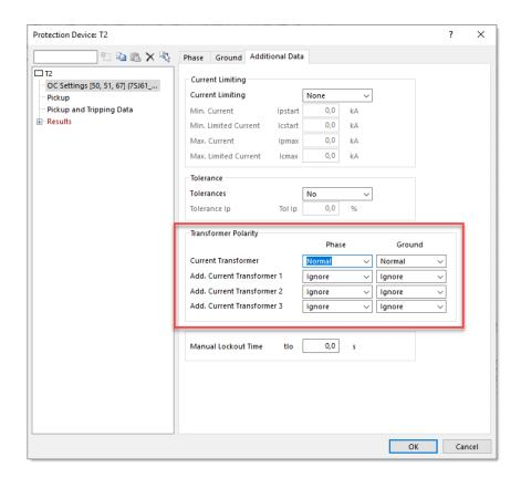
The currents are added on the secondary side for each phase in the protection coordination. This is added irrespective of the conversion ratio of the transformers but a warning is output if the conversion ratio is not the same.
